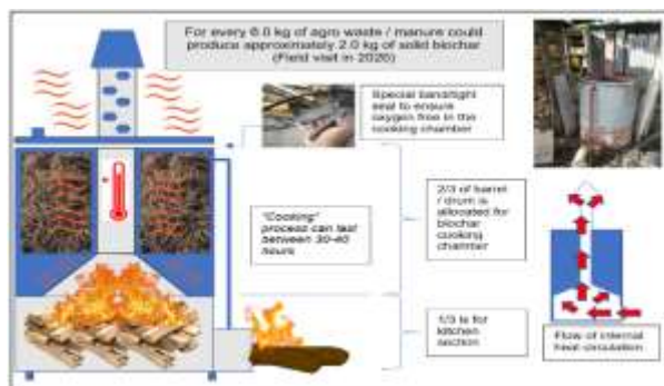
Fig. 2. Cross section of biochar kitchen that used by smallholders in Hulu Terengganu.
