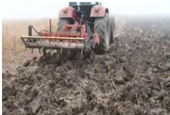
Fig.2. Execution of scarifying and rolling work
