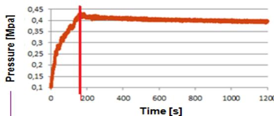
b) Changes to the average values of surface pressures during creep test
