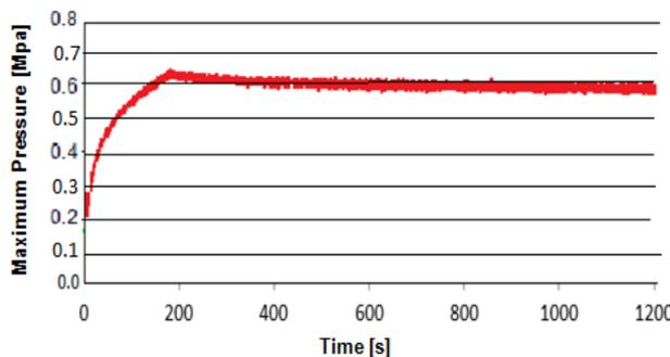
Fig. 5. Changes to the average values of surface pressures during creep test
