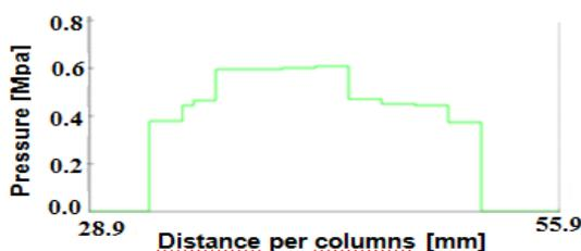
c) Distribution of surface pressures in A-A cross-section
