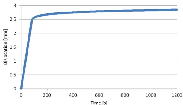
Fig. 3. The progress of the creep process
