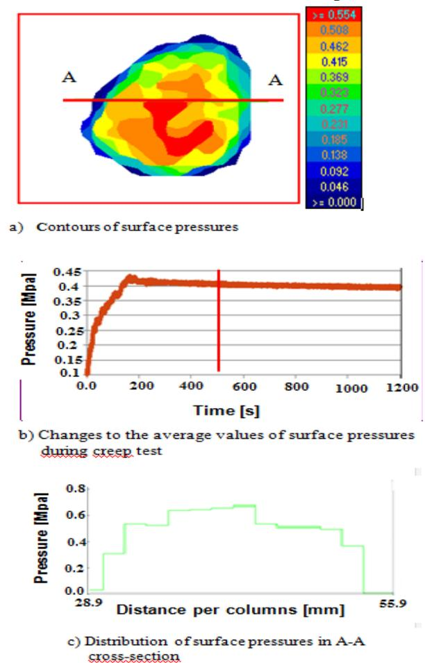
Fig. 7. Contours and distributions of the average values of surface pressures ka  $\Delta t=500\text{ sec.}$
