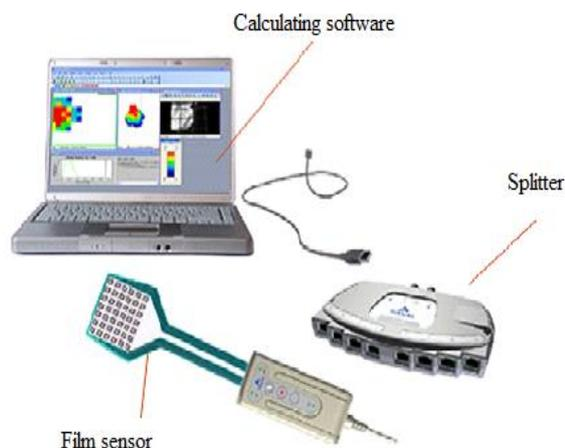
Fig. 1. Tekscan measuring system
