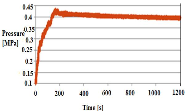
Fig. 4. Changes to the average values of surface pressures during creep test
