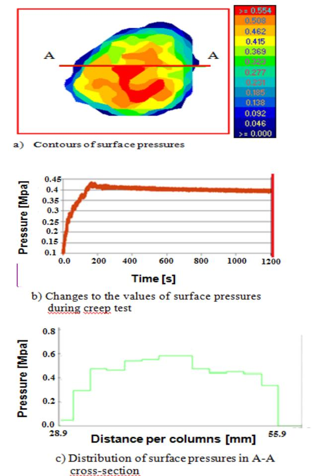
Fig. 8. Contours and distributions of the average values of surface pressures ka  $\Delta t=1200\text{ sec.}$
